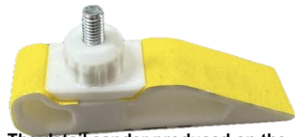
The detail sander produced on the 3D printer
