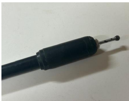
The home-made texturing tool using the cut off end of an old flexible shaft from a rotary tool with a round burr used for texturing.
