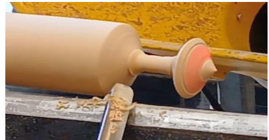
The top was textured, coloured and waxed before cutting off with a skew and moving on to the next top.
