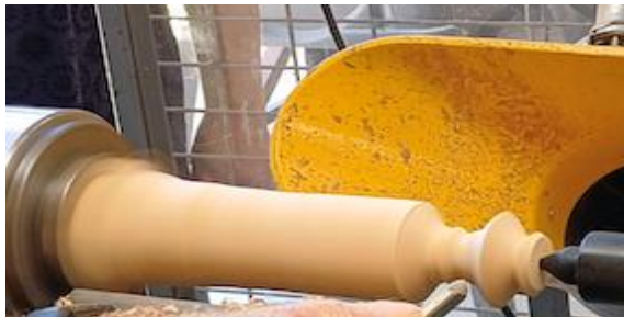
Roughing gouge was used in a planning mode to finish rounding the stock and then a spindle gouge to shape the top.
