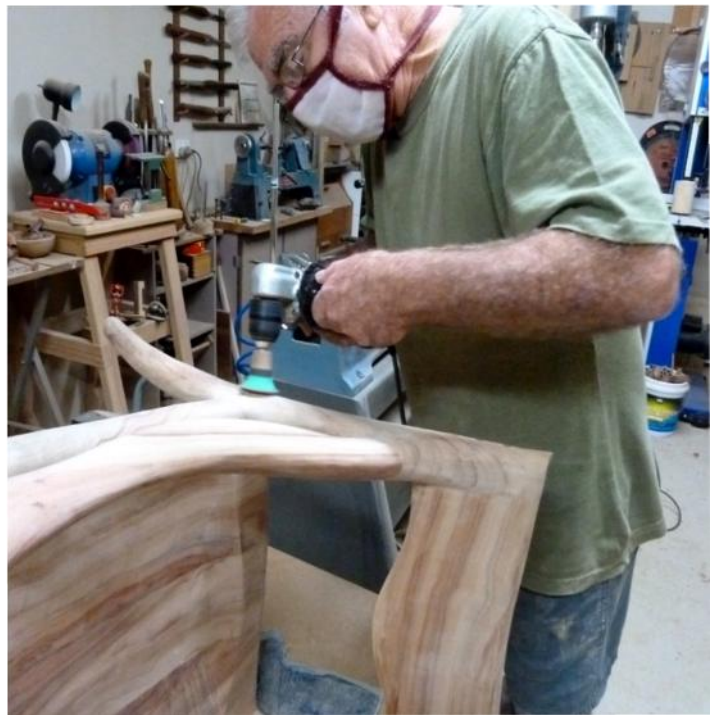
Power sanding through the grits and then by hand with finer grits.
