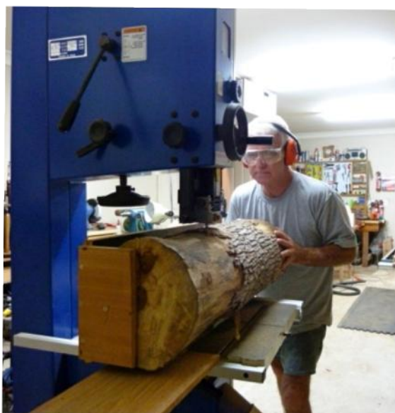
Managed to mill and size the camphor with the assistance of jigs.
