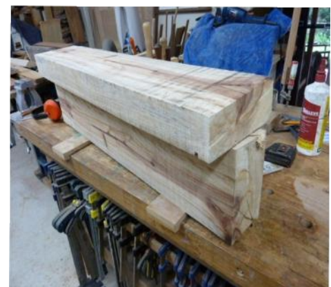
Managed to mill and size the camphor with the assistance of jigs.
