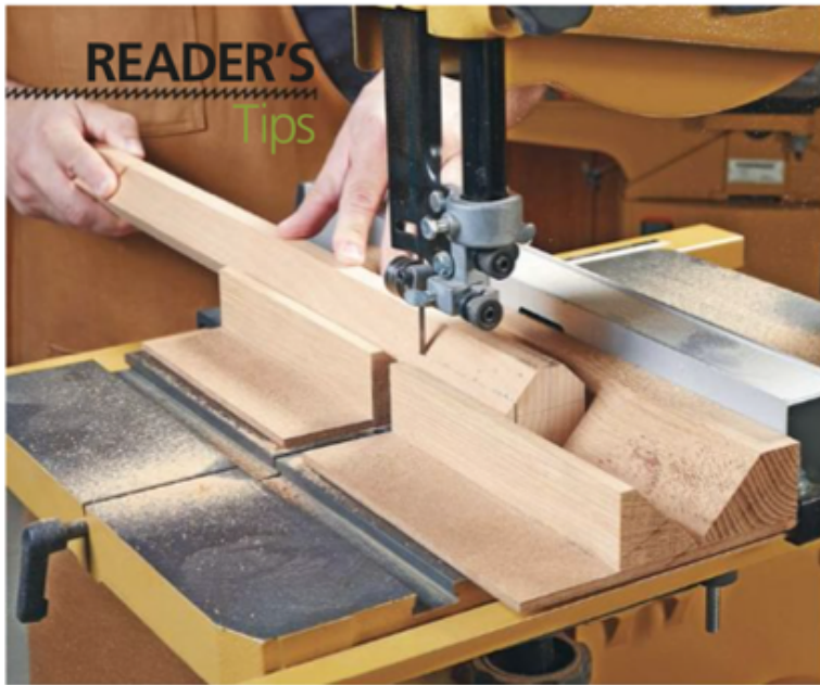
▲ The V-jig works well for any odd shaped pieces, such as when notching or ripping dowels.
