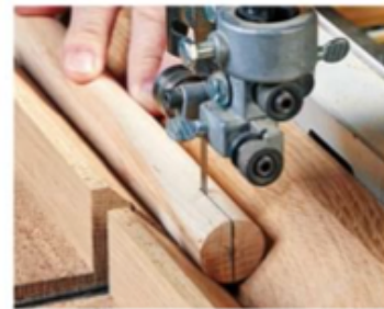
▲ The V-jig works well for any odd shaped pieces, such as when notching or ripping dowels.
