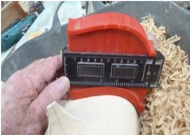
Checking the consistency of the curve profile
