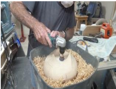
Final sanding from 150 to 600 grits to achieve the final finish
