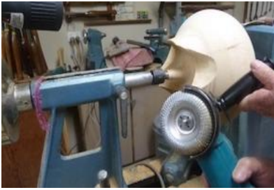
The legs shaped out with a 100mm tungsten chip disk in an angle grinder
