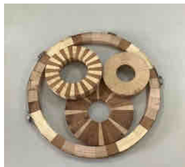
Bob Longlands had some examples of segmentation using a purpose made jig.
