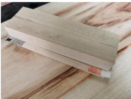
Fig 1 – Four square blocks glued up using paper glued joint
