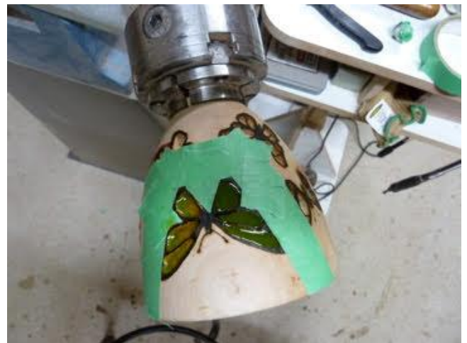
Masking the areas for resin infill.
