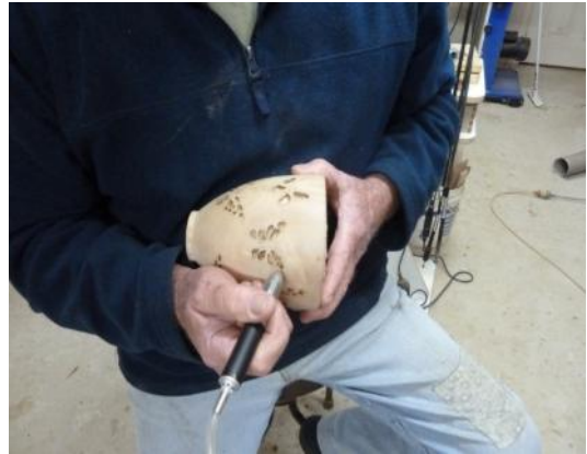
Piercing/carving voids to be filled with coloured resin
