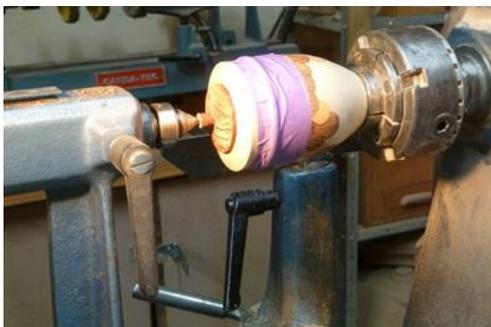
Box with the lid tapped back on for turning and further drilling and the inserting of additional plugs
