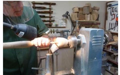
Turning out the box exposing the plugs on the inside
