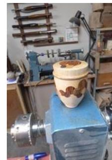
The completed box prior to the shaping of three small feet and finishing in a satin lacquer
