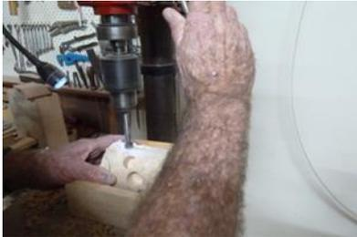
Drilling holes with a forstner style bit
