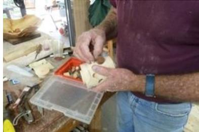
Inserting selected plugs in various timbers
